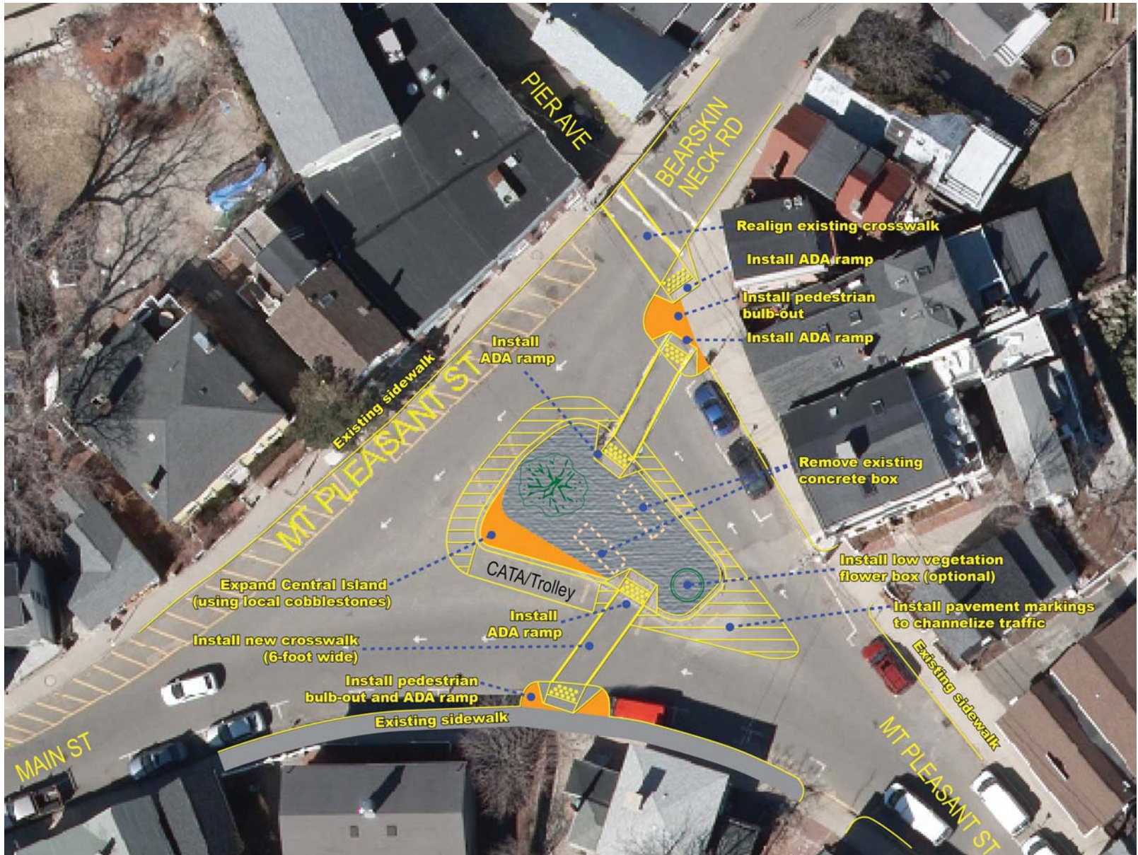
Proposed Improvements Alternative 2: Expand Central Island and Install Crosswalks and ADA Ramps
