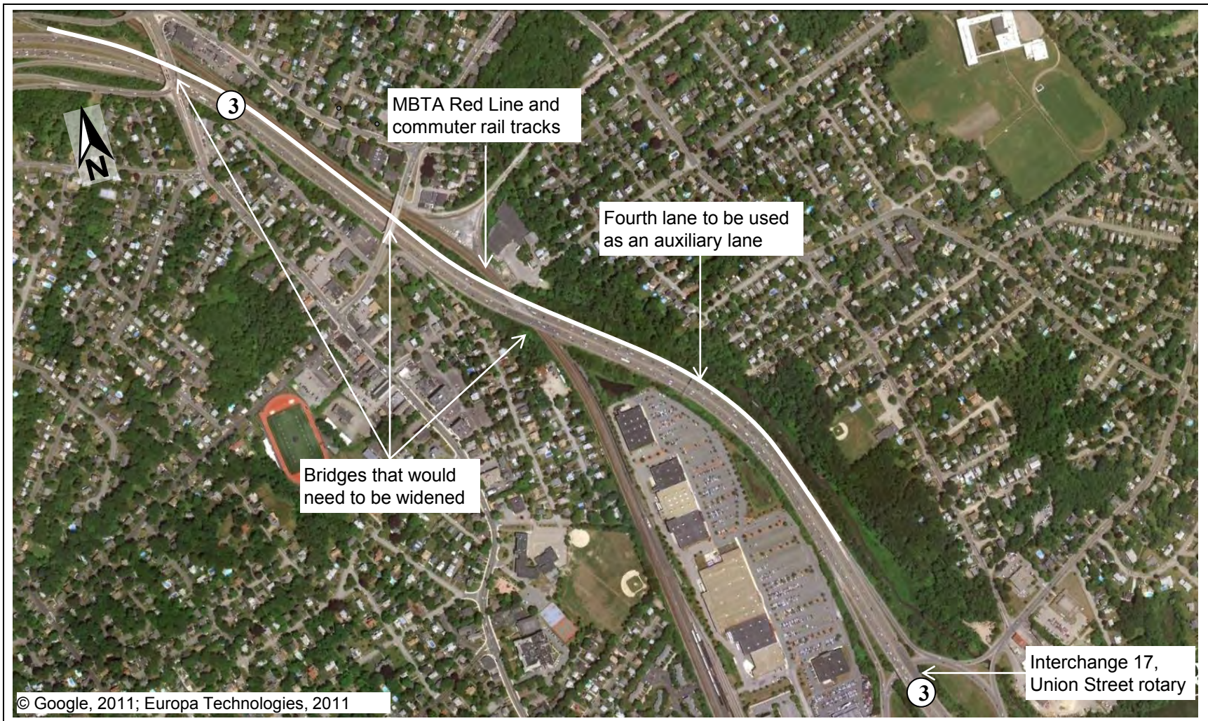
FIGURE 14B Alternative 2: Add an Auxiliary Lane (Fourth Lane) on Route 3 Northbound between Interchanges 17 and 19
