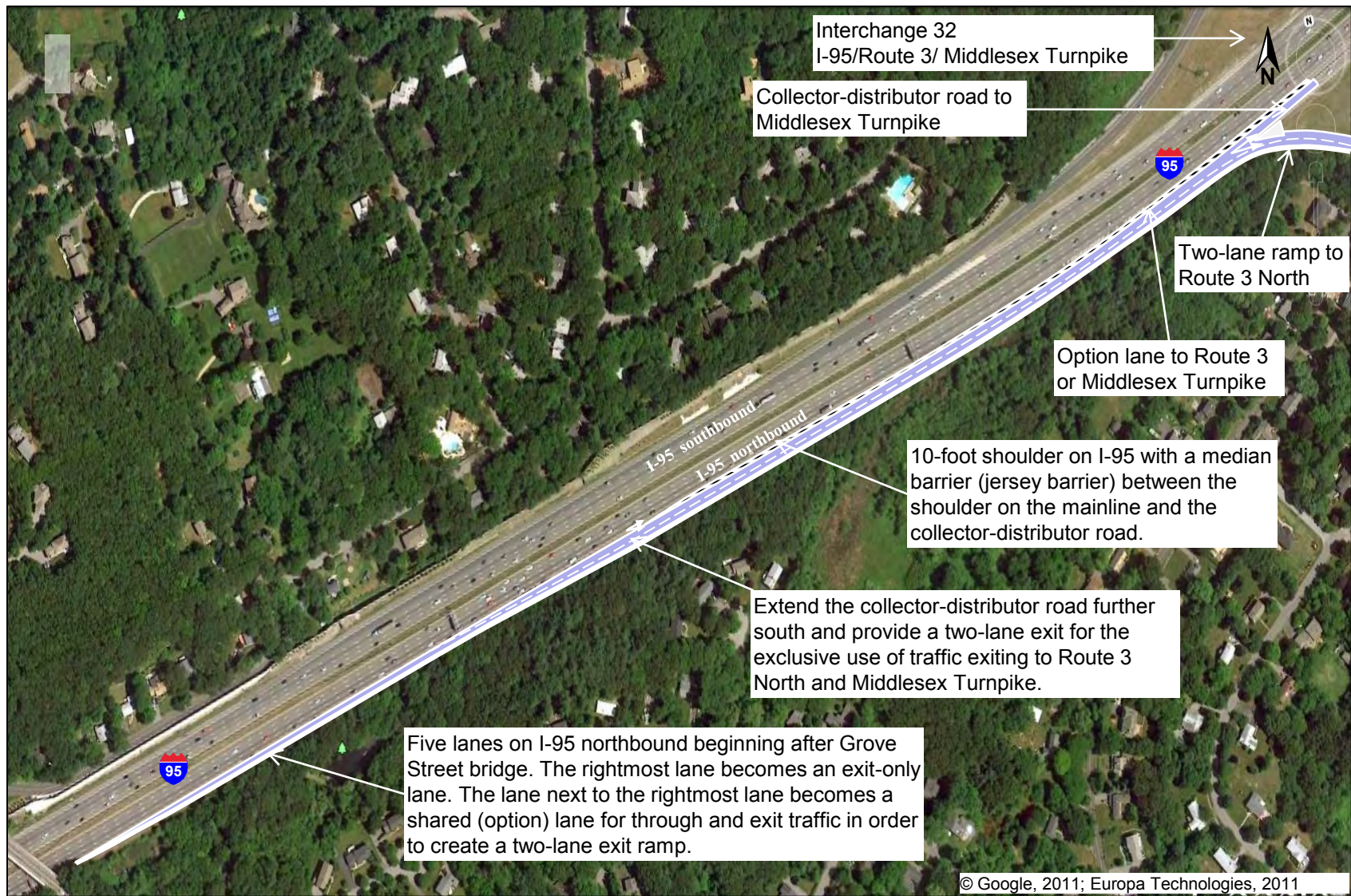
FIGURE 20 Construct a Two-Lane Exit Ramp for Traffic Exiting I-95 Northbound to Route 3 and Middlesex Turnpike
