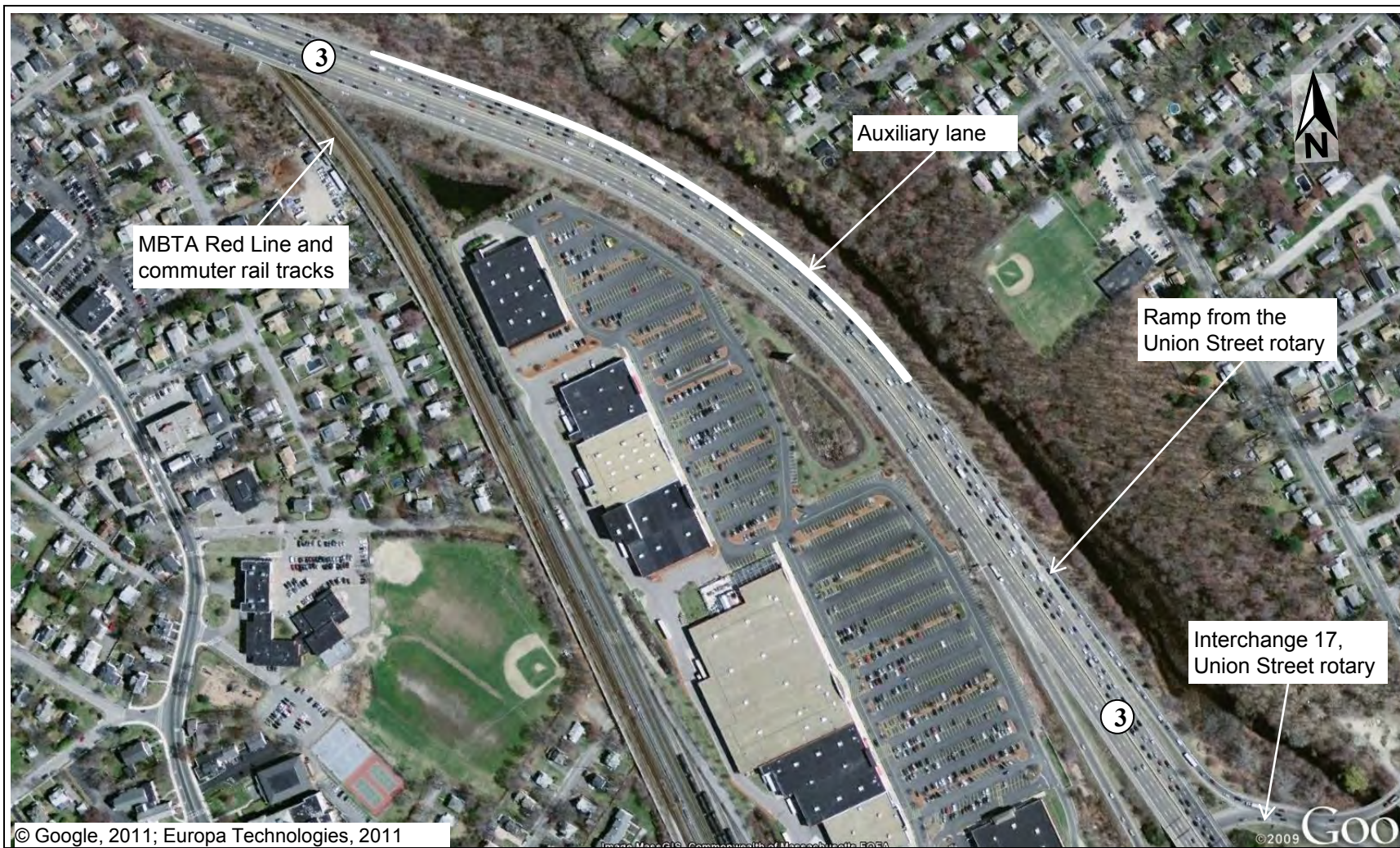
FIGURE 14A Alternative 1: Use a Short Section of the Right Shoulder as an Auxiliary Lane on Route 3 Northbound
