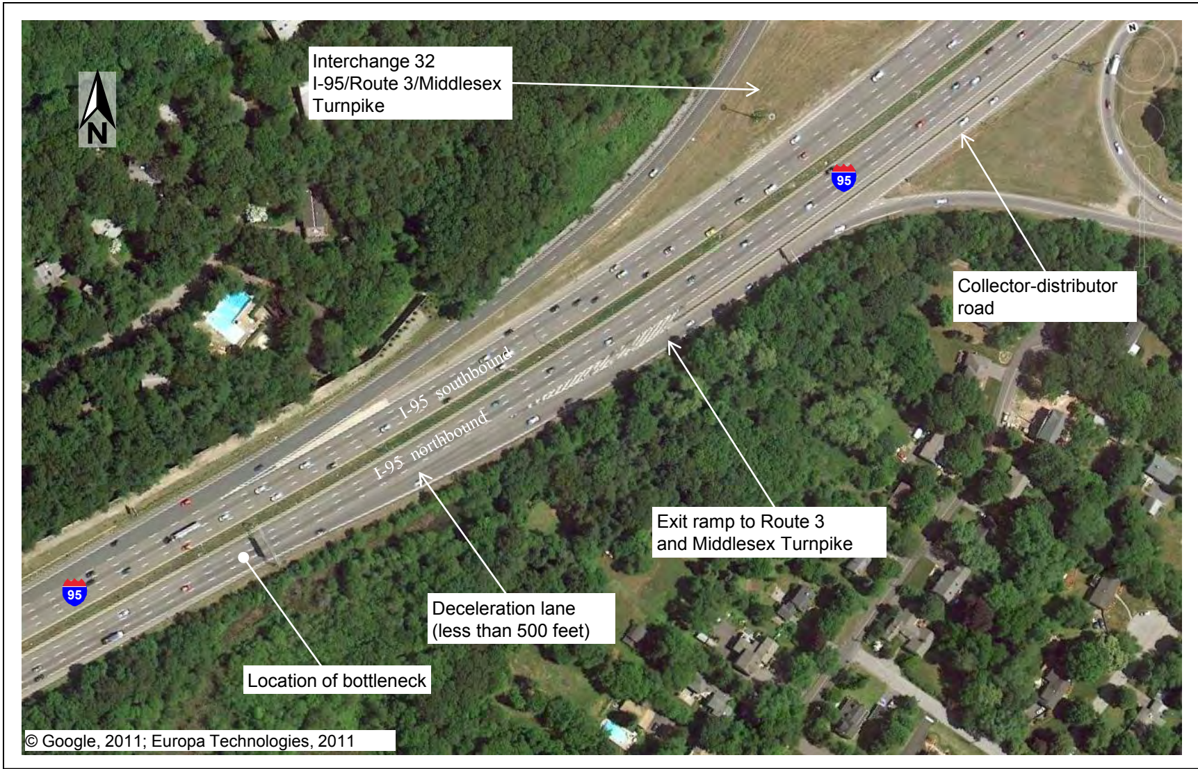
FIGURE 15 Location of Bottleneck and Configuration of Ramps at Interchange 32 in Burlington
