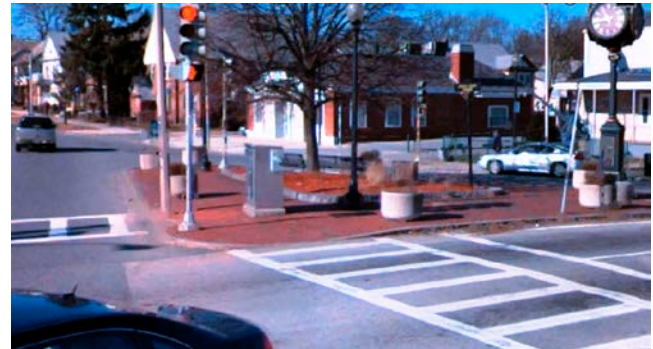
Gallivan Boulevard and Granite Street/Adams Street: Choke points that narrow the effective sidewalk width, such as mailboxes, utility poles and equipment, and landscaping.
