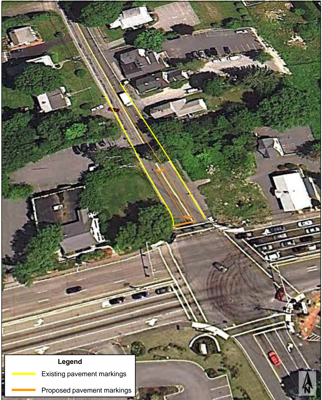
FIGURE 5 Proposed Restriping of Central Street
